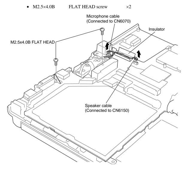
Figure 4-36 Removing the system board (1)
